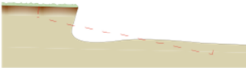
Figure E1: Headcut cross section and the battering profile (red)
