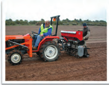
Photo 5. The Grassy Groundcover Research Project seeder was developed to sow a complex mix of grassland species onto a weed free soil surface. This is a modified turf seeder originally designed for sowing golf courses and the like.
