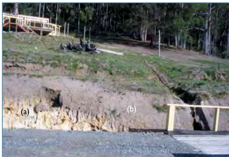
Figure 13. The severity (or sodium content) and depth of dispersive subsoils can vary considerably over short distances. (a). At this site highly dispersive subsoils exist meters away from (b) non-dispersive soils.
