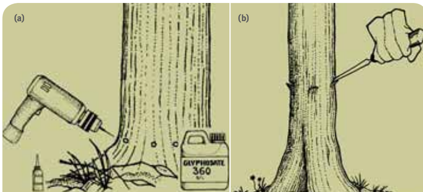
Figure 10.1: Stem injection (a) and frilling (b). Illustrations: Norman Yeend and Virginia Bear.
