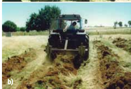
Figure 15.6: a) A tractor-mounted ripper-moulder showing ripping arm and mounding discs. b) Ripped and mounded soil after one pass. Some applications will require two passes. Photos: D. Carr
