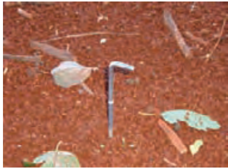
A line on an erosion pin shows the original soil level.
