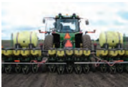
This John Deere precision planter uses a coulter and tine mechanism.
