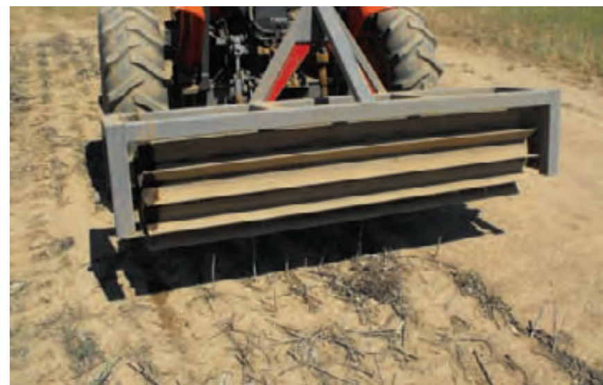
A crimp roller can reduce the need to cultivate for weed control.
