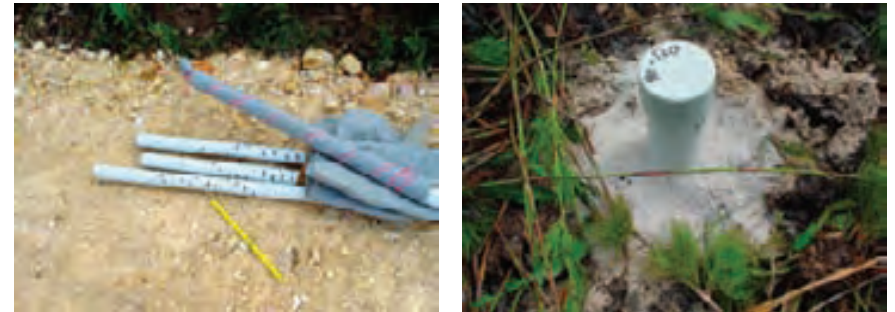
Slotted pipes for use as piezometers. In the ground only the top of the pipe is visible. Source: Keith Bolton
