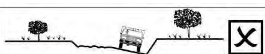
Figure 3—Subsurface roads (not recommended)
