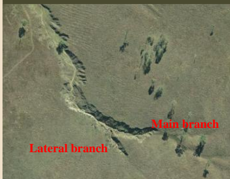
Aerial image showing main and lateral branches of an active eroding gully.
