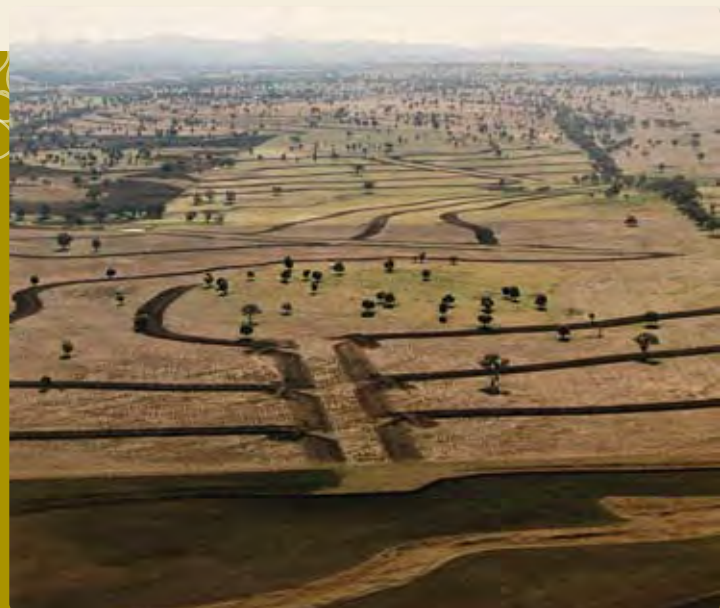
PHOTO 9 Erosion control earthworks and stubble retention on Class 3 land, protecting soil from raindrop impact, sheet erosion, rilling and gullies near Tooraweenah. (Chris O'Brien)
